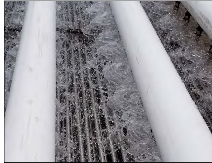
Figure 7. Nozzle Spray Pattern
