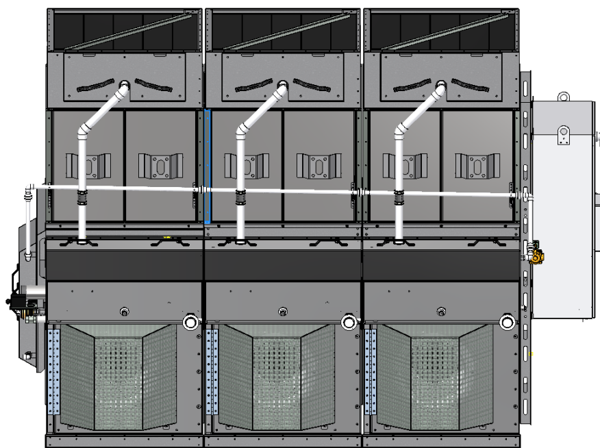
Figure 53. Crossover piping installed
