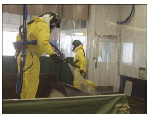
TriArmor® Corrosion Protection System Spray Booth
