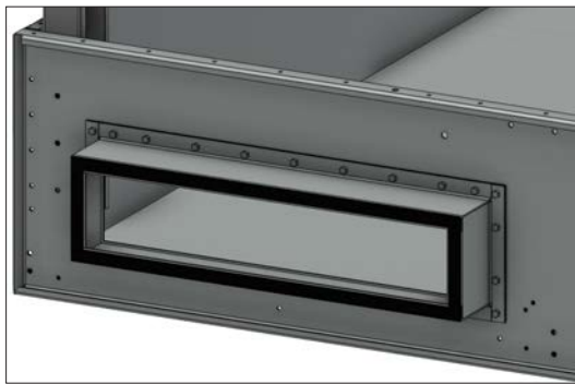
Figure 5. Flume Box Butyl Sealer Tape Application
