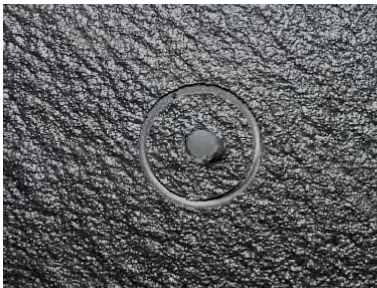
Figure 73. Scored TriArmor® Corrosion Protection System
