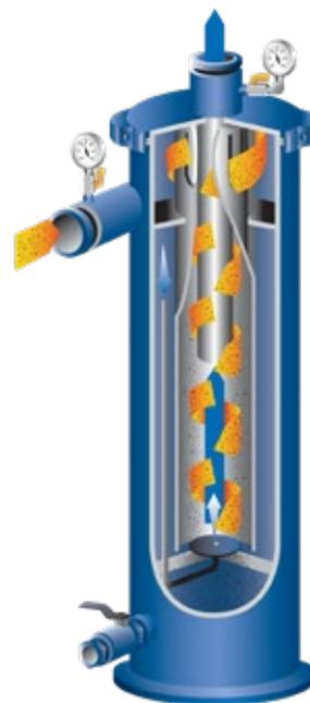
Figure 6. Centrifugal Separator Principle of Operation
