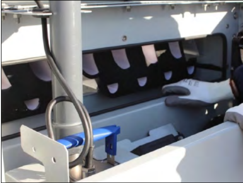
Figure 22. Water Diverter Inspection Panel
