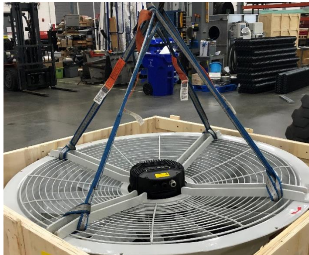
Figure 29. Fan and Motor Assembly Lift
