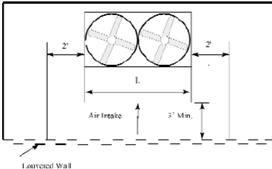
**Figure 4: Plan view of single air intake unit in enclosure with louvered walls**
