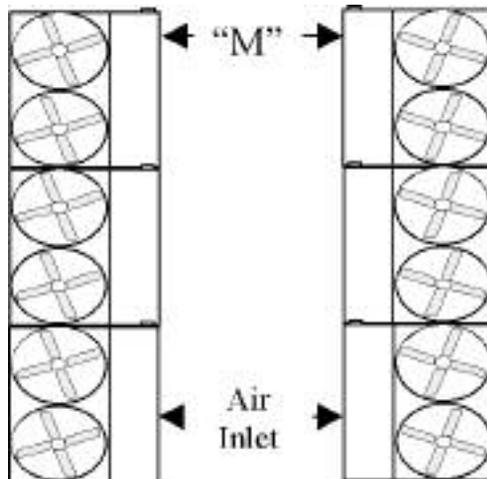
**Figure 6: Plan view of multi-cell units with air intakes facing each other**
