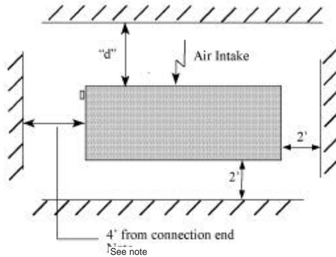
**Figure 1: Plan view of recommended unit servicing and maintenance spacing for single air inlet unit Series V Cooling Towers, Closed Circuit Cooling Towers and Evaporative Condensers**
