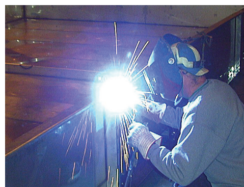
Welded Type 304 Stainless Steel Cold Water Basin
