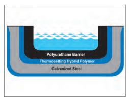
TriArmor<sup>®</sup> Corrosion Protection System Triple Layer Protection of the Cold Water Basin
