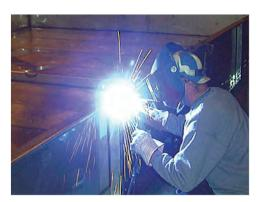
Welded Stainless Steel Cold Water Basin
