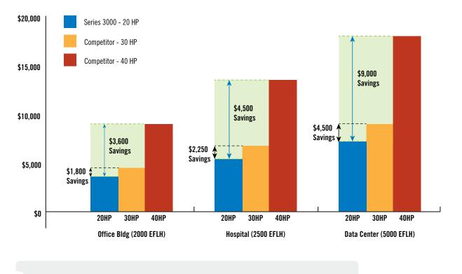
NOTE: Energy Cost Savings Based on a 400-Ton System (\$0.12 kWH) for equivalent full load hours (EFLH).
