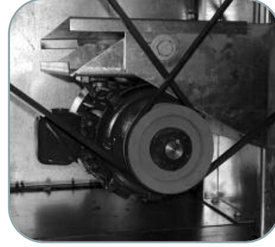
Figure 7 - Adjustable Motor Base FXT Models 160-257 and 320-514
