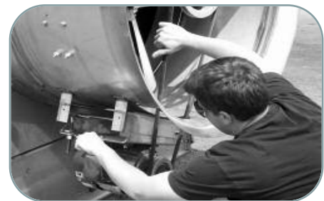
Figure 3 - Fan Belt Adjustment
